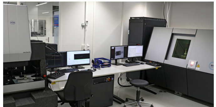
The heart of Maxon's metrology department: the Video-Check HA 3D CNC multisensor coordinate measuring machine (left) and the Tomoscope S computed tomography coordinate measuring machine (right). An additional offline workstation allows CT data to be evaluated in parallel with measurements taking place at the same time. © Werth Messtechnik
