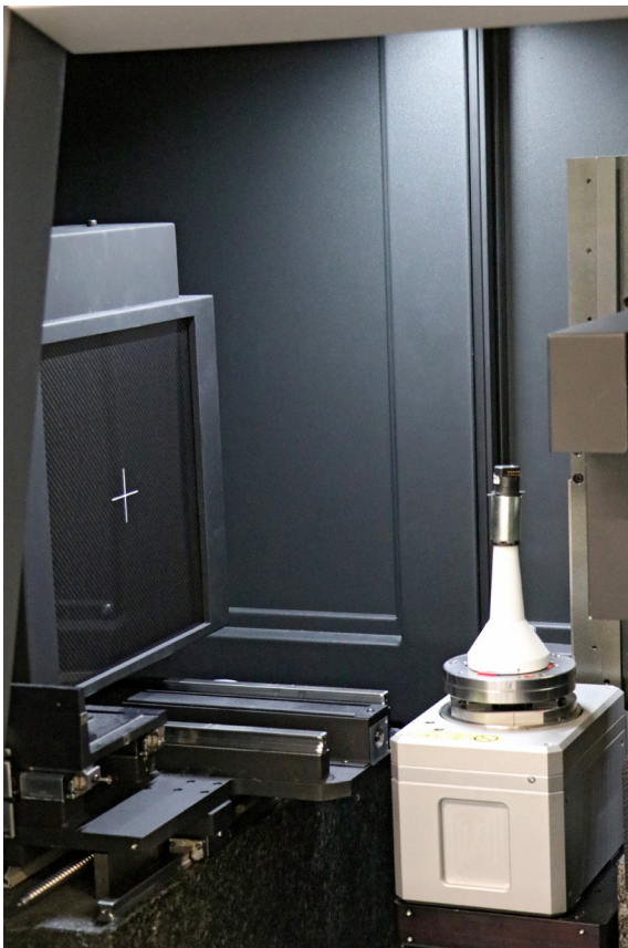
Maxon uses the Tomoscope S, among other things, to X-ray complete motors and visualize all internal components. © Werth Messtechnik
