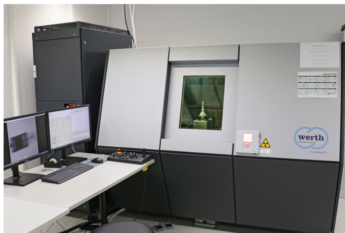
The Werth Tomoscope S is suitable for visualizing and highly accurate measurement of workpieces and assemblies made of different materials. © Werth Messtechnik
